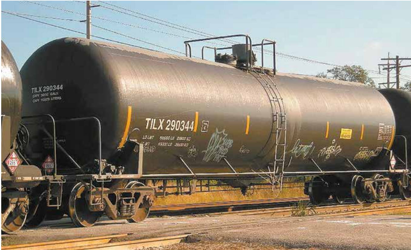
A DOT-111 tank car is the vehicle of choice for transporting crude oil from fracking fields to the coasts. The cars also carry other volatile substances, like ethanol, and can be spotted daily in the Erie area.
